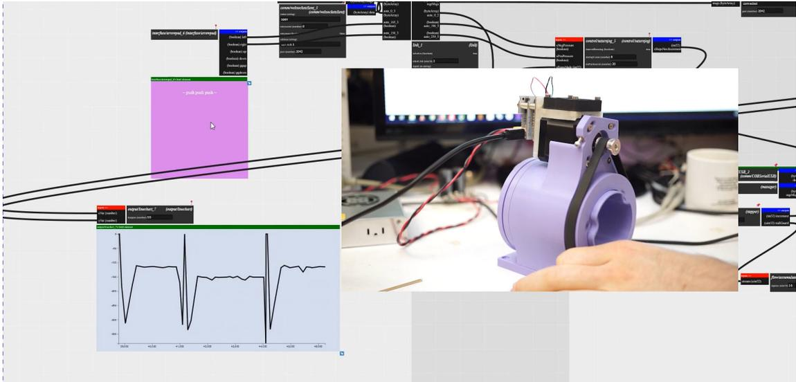
Figure 6-5: Here I visualize torque feedback from this rotary device in real-time, by routing an heuristic torque measurement (approximated with back-EMF sensing) output from the stepper driver into the browser, where they are plotted. The spikes in this chart were generated as the rotary device accelerated through direction changes.
