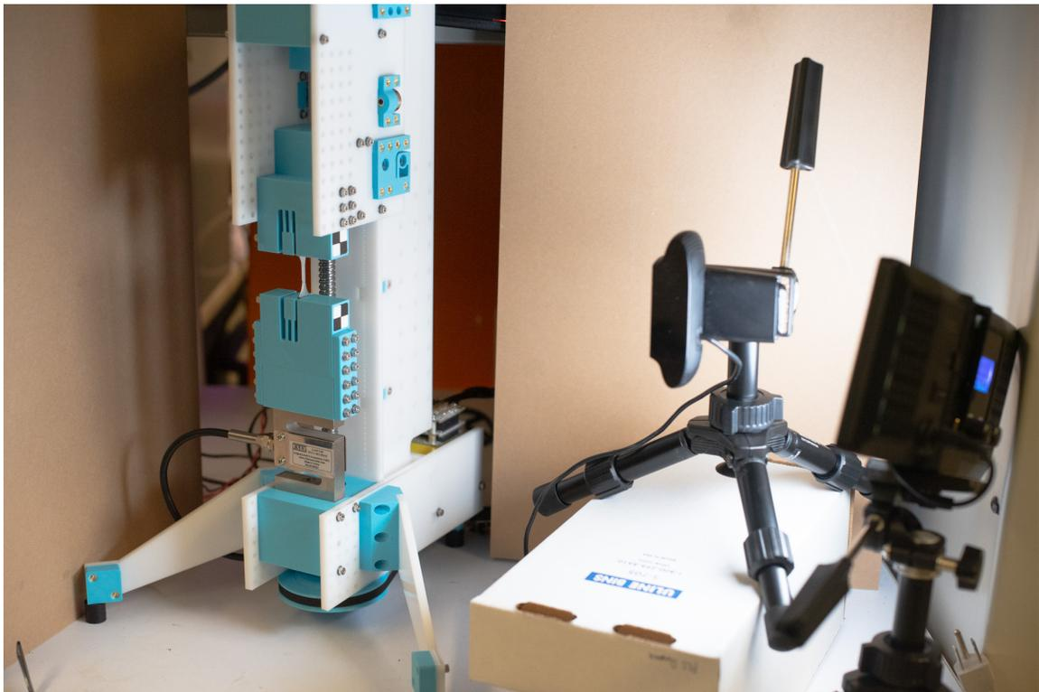
Figure 6-6: A small Stress and Strain measuring machine, using computer vision displacement measurement.
